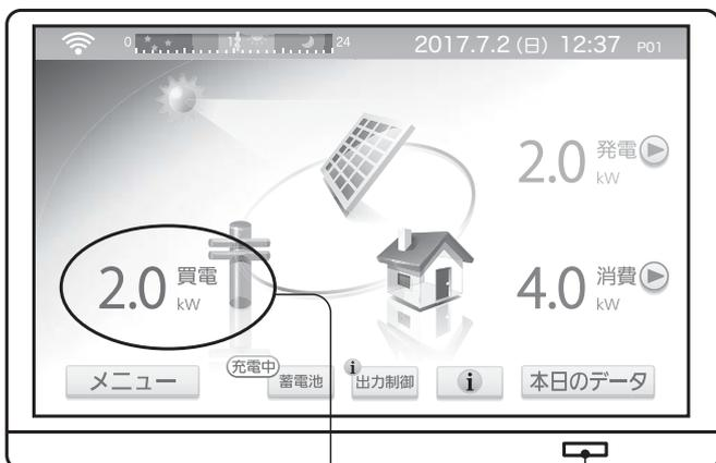
The smart meter display shows a central house icon with a solar panel. To the left, a red circle highlights '2.0 買電 kW' (2.0 kW power purchased). To the right, it shows '2.0 発電 kW' (2.0 kW power generated) and '4.0 消費 kW' (4.0 kW power consumed). At the bottom, there are buttons for 'メニュー' (Menu), '充電中 蓄電池' (Charging battery), '出力制御' (Output control), 'i' (Info), and '本日のデータ' (Today's data). A red indicator light is shown at the bottom right.
